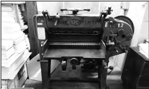
A 1950's Vintage Victory-Kidder Printing John Perfecta Guillotine machine. Used for cutting and trimming paper, cardboard, and other print materials with high precision. Still in use here at the Voice.
