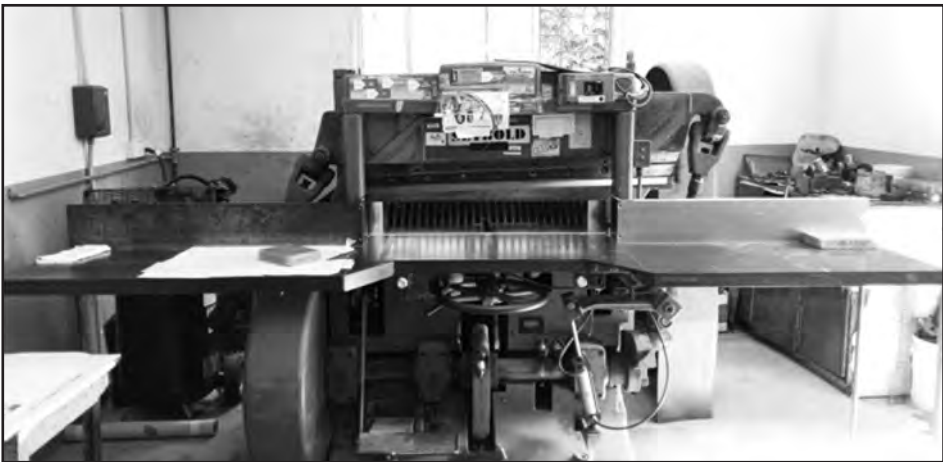
The Harris Seybold CFB Paper Cutter is a guillotine-style cutter used for making straight cuts through single sheets or stacks of paper. It was manufactured by Charles Seybold starting in 1888 in Dayton, Ohio. Due to their size and strength, these cutters are still used in the printing industry and in manufacturing
