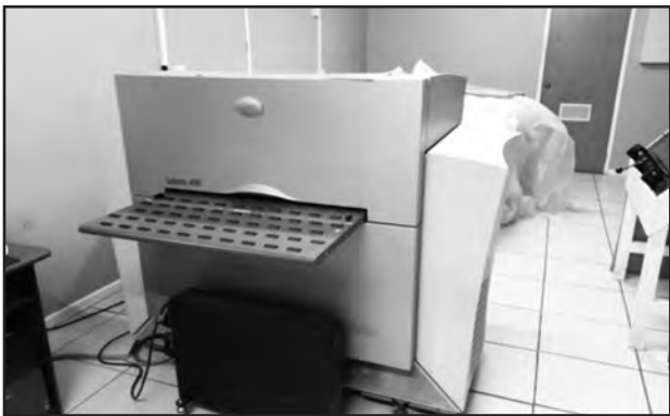
The Lotem 400 is a plate setter that uses thermal imaging technology to produce high-resolution images. It was manufactured by Creo, Kodak in Canada
