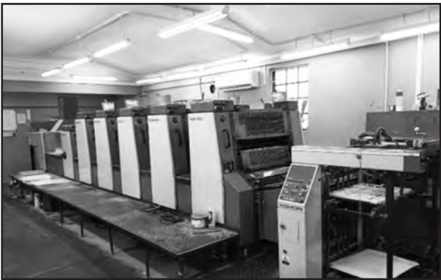
The Komori Lithrone 26 press is designed to deliver high-quality, efficient printing for a range of commercial products such as brochures, catalogues, flyers, periodicals, and packaging materials. Their advanced features and automation capabilities make them ideal for high-demand printing environments
