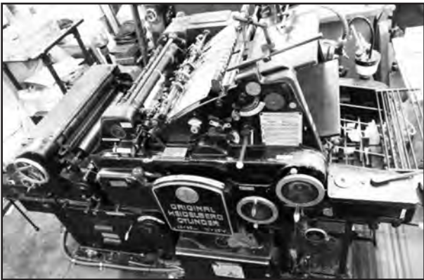
A Heidelberg Original Cylinder printing press, which is a well-known letterpress machine used for high-quality printing, die-cutting, embossing, and numbering. This type of press is valued for its durability and precision in speciality printing tasks
